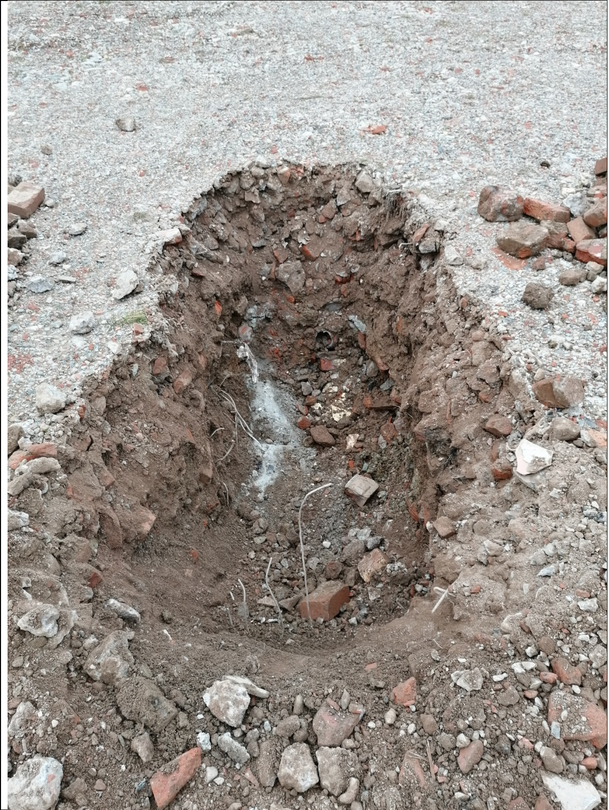
Plate 9: TP105 terminated at a depth of 1.00m
