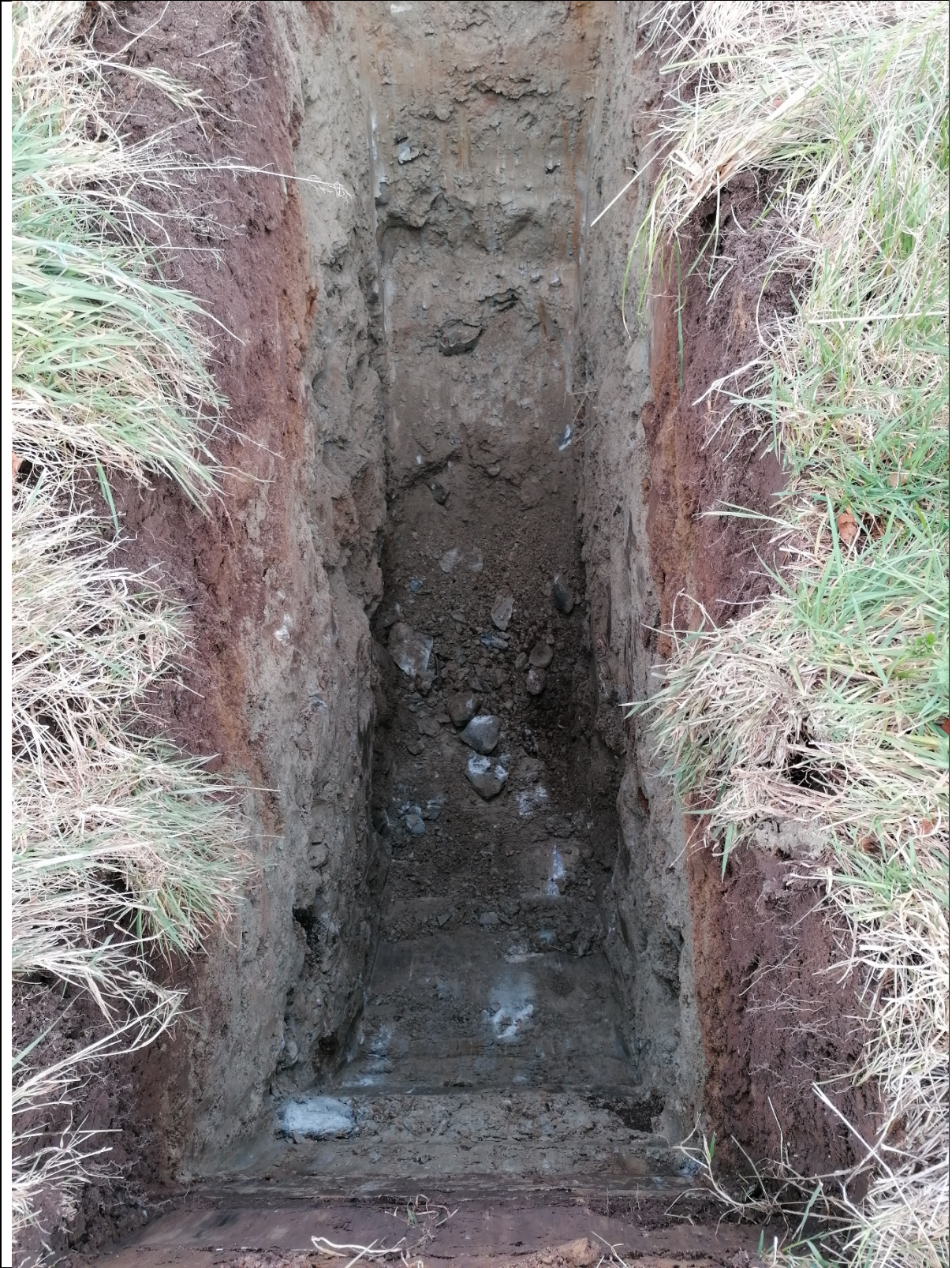
Plate 3: TP102 terminated at a depth of 2.50m
